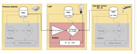
Figure 2: Light, presence sensor, daylight sensor example model.
