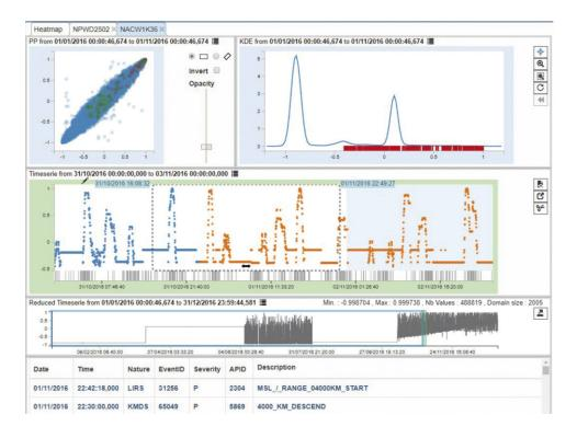
Figure 1: DMSS provides a dashboard to show telemetry data coming from remote sensors.
